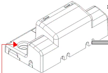
Mounting Bracket: Provision has been made for two screws that may be used to secure the bracket to the mounting surface.
