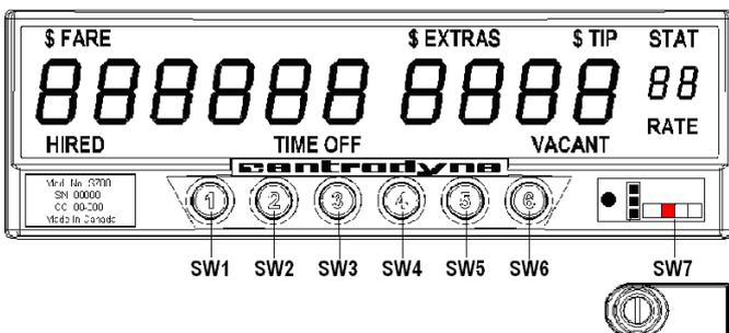
**VACANT:** The taximeter is normally in the Vacant state. If required, press switch 6 to select rate. Press switch 1 (SW1) to Hire taximeter.
